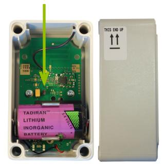
Once the beacon is mounted to a desired position it can be turned on by inserting the jumper. Once the jumper is connected, the beacon is operational. The LED will blink on transmission interval. If the beacon is in configuration mode it will blink in 2 seconds interval with two colours.
