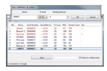
When the "Keep on config mode" box is ticked, all beacons in configuration mode (marked in bold on the list) remain in the configuration mode 10 minutes also when outside the configurator coverage area.
