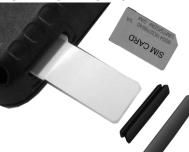
1. Slide the SIM card to the holder from the hole on the side of the unit slightly tilting the SIM card towards the keyboard when pushing it in. Contacts in the SIM are facing towards keypad and the cut corner of the card outward. Use the
