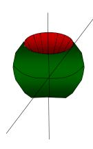
Tilt angle e.g. 45° Allowed orientation in green. Both on top and bottom. If filted more than 135 degrees, again in allowed orientation. Alarm when in RED area NOTE, that also movement condition must be met
