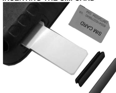
1. Slide the SIM card to the holder from the hole on the side of the unit slightly tilting the SIM card towards the keyboard when pushing it in. Contacts in the SIM are facing towards keypad and the cut corner of the card outward. Use the silver tape in the salesbox to assist if you need to remove it or inserting to SIM holder is difficult. **Do not use force as the SIM will go to its place easily.**
