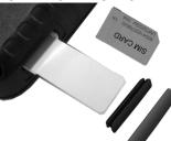
1. Slide the SIM card into the holder from the hole on the side of the unit. Contacts in the SIM are facing towards keypad and the cut corner of the card outward. Use the silver tape in the sales box to assist if you need to remove it or inserting to SIM holder is
