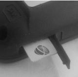
1. Slide the micro-SIM card to the holder from the hole on the side of the unit contacts in the SIM are facing towards keypad and the cut corner of the card inward. Make sure the card locks to holder. **Do not use force, as the SIM will go to its place easily**. 2. Push the SIM card all the way in with e.g. another
