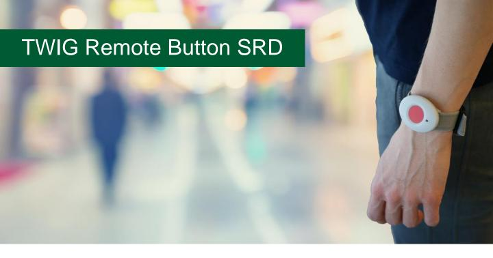
TWIG Remote Button is a short range device of SRD transceiver category 2, designed to be worn on the neck, on the wrist or in the pocket. Paired with a nearby SRD or SRD3 -enabled TWIG personal alarm device as its base station, it enables remotely launching MPTP protocol messages with a single push of button.
