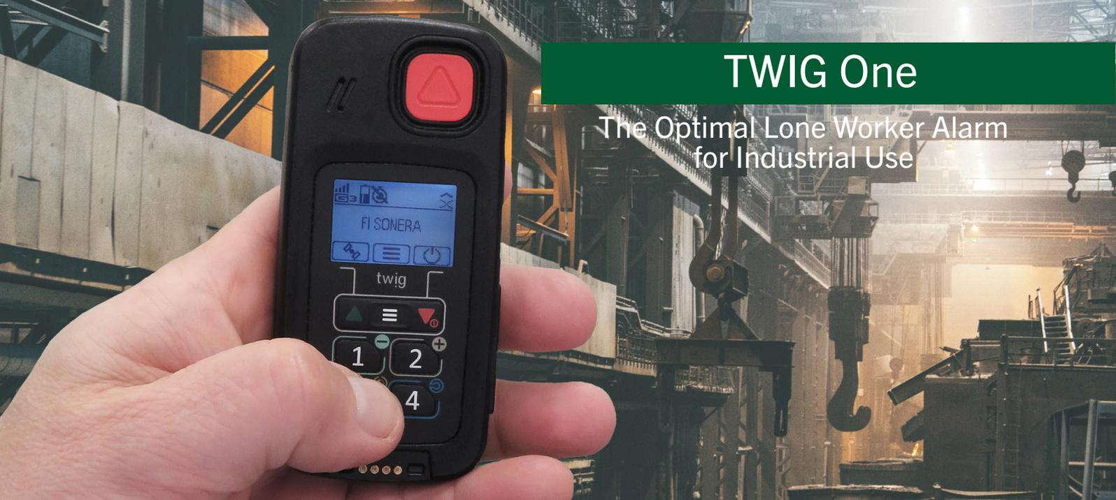
TWIG One is a personal alarm device optimized for lone worker safety in noisy and hazardous industrial environments. The essential lone worker protection functions, powerful loudspeaker, robust design, preprogrammable device keys, configurable user interface, compatible accessories, scalable functions and easy integration with various monitoring systems make it a serious choice for the requirements of industry.
